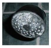
On the left is a photo of the showerhead in the left hand cubicle of the women's locker room on October 1<sup>st</sup>, 2009. The scale on the showerhead was hard and encrusted and could only be removed by using an acid cleaner.
